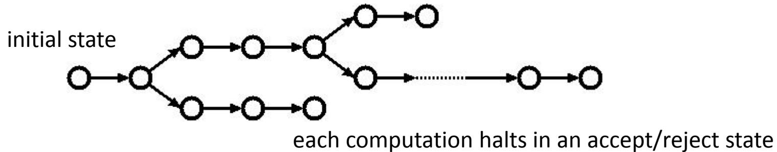
An  $\text{NP}$  problem  $L$  is recognized by a nondeterministic Turing machine in polynomial time. That is, there is a computation path to an accept state of length polynomial of  $n$ .
