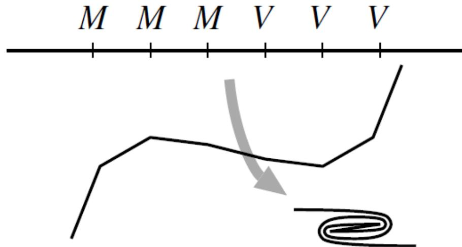
The way of folding is **unique** by bit longer end-edges
