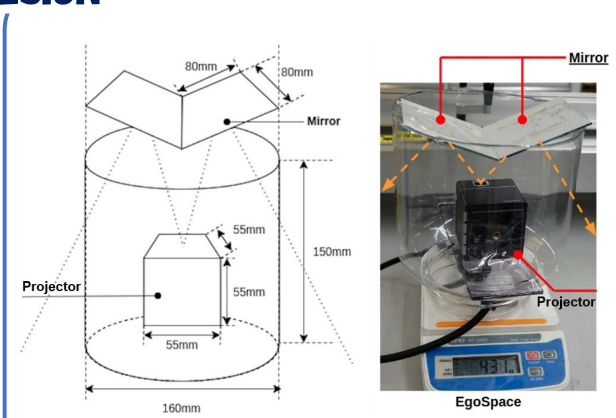
Design blueprint of the proposed device (left) and our developed prototype (right)
