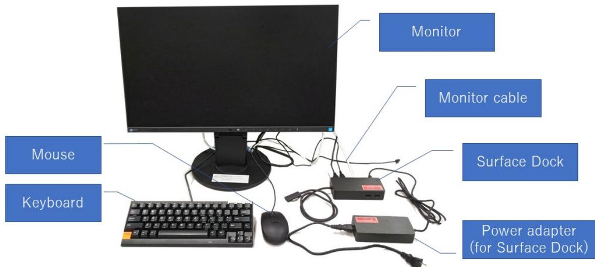
Installed equipment (with surface dock) is the above devices.
