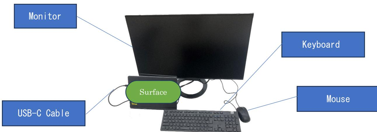
Installed equipment (without surface dock) is the above 4 devices. Please connect the Surface to the monitor with a USB-C cable as shown in the picture. By connecting the Surface and monitor with a USB-C cable, you can use the screen output and the USB-A port on the monitor side.
