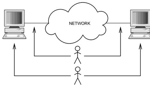
Figure 1. Observing end-to-end application performance, and measuring the quality degradation in the network.
