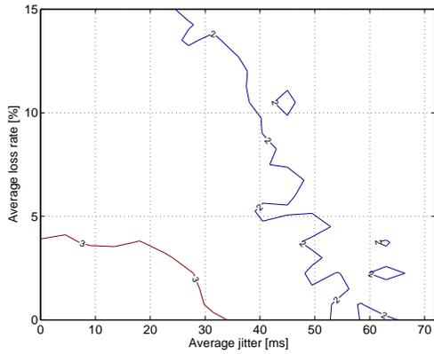
Figure 4. Contour plots of the boundaries between quality levels for the G.726 codec.
