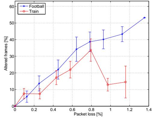
Figure 8. Number of altered frames as function of packet loss.
