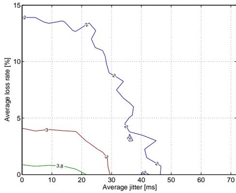
Figure 3. Contour plot of the boundaries between quality levels for the G.711 codec.
