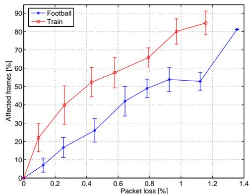
Figure 10. Number of affected (altered or dropped) frames as function of packet loss.
