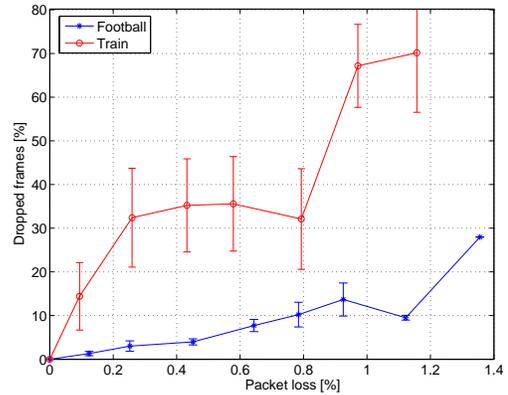
Figure 9. Number of dropped frames as function of packet loss.
