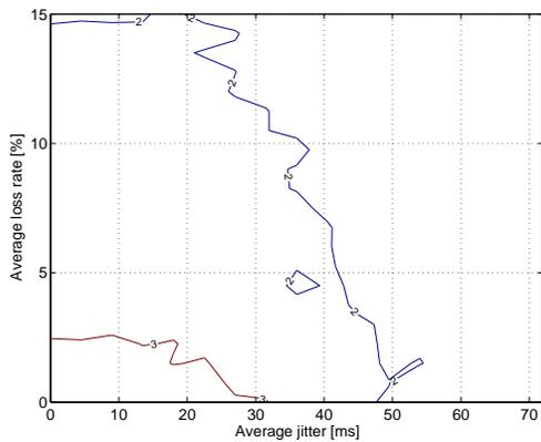
Figure 5. Contour plot of the boundaries between quality levels for the GSM codec.
