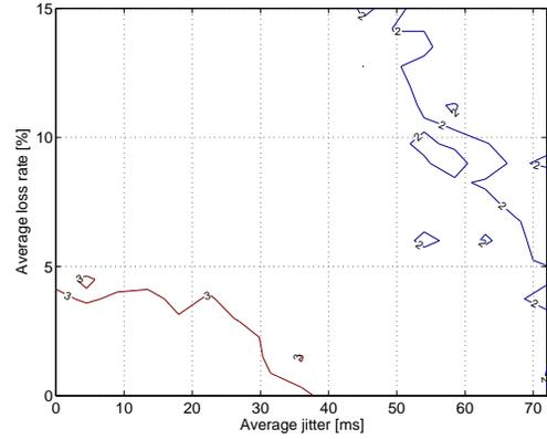
Figure 6. Contour plot of the boundaries between quality levels for the G.729 codec.
