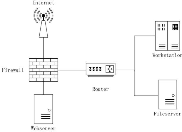
Figure 8. Network topology for the experiment scenario.
