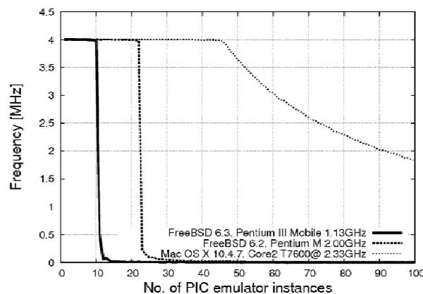
Figure 3. PIC emulator frequency accuracy depending on the number of executed instances
