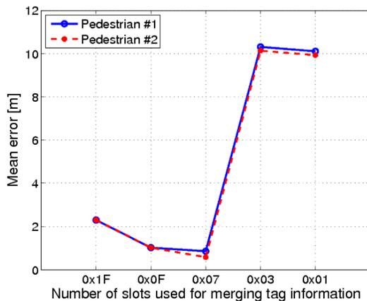
Figure 3. Mean localization error versus of the number of time intervals used for merging tag information.
