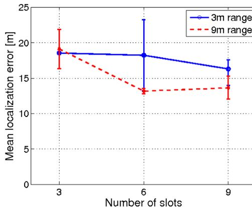
Figure 2. Mean localization error versus the number of slots used in time-multiplexed communication.
