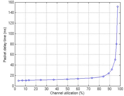
**Figure 3. Packet delay time as a function of channel utilization**
