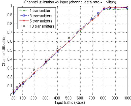
**Figure 2. Channel utilization as a function of input traffic**
