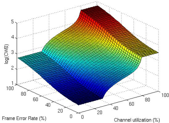
**Figure 6. CWB routing metric as a function of channel utilization and FER**
