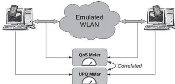
Figure 2: WLAN emulation for application performance assessment.
